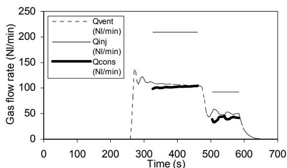
Figure 2 Experiment 3a at 70 bar and 7.2 °C. Methane gas. The gas injection rate was changed after about 460 seconds.
