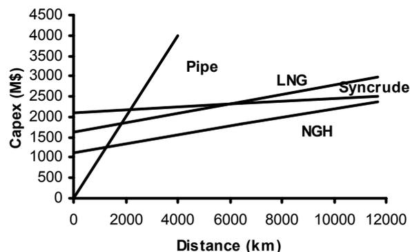
Figure 1 Approximate capital cost with transport distance, dry-hydrate case.
