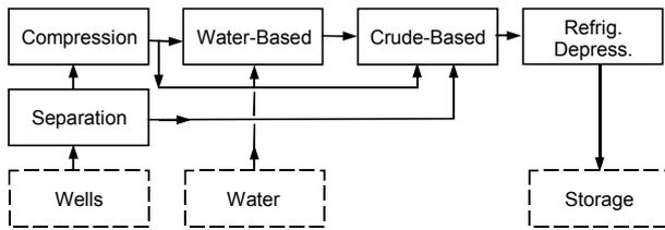
Figure 3 Main units of a hydrate slurry process.
