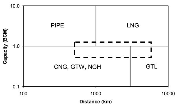
Figure 5 - Capacity-distance diagram (BCM per year versus km).
