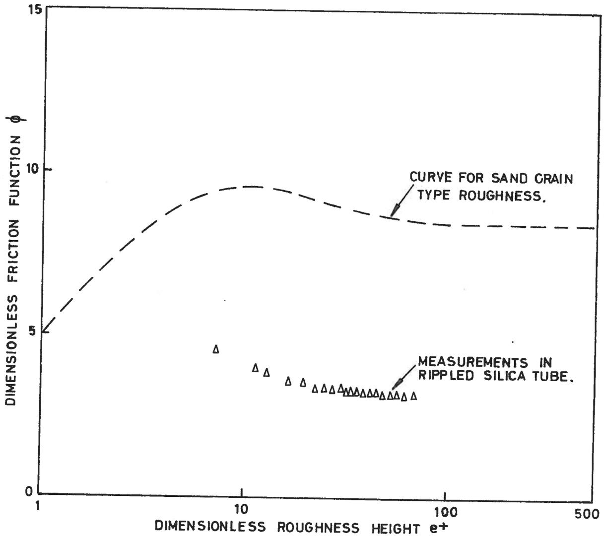
A.E.R.E. R.8703. FIG.9. FRICTION FUNCTION FOR TUBE WITH RIPPLED SILICA DEPOSIT.
