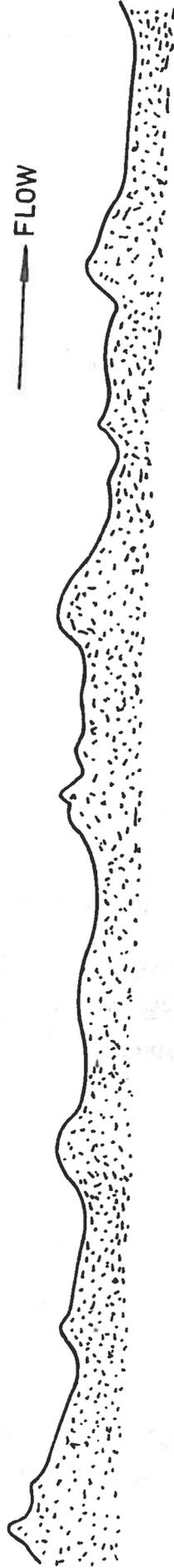
(b) PROFILE OF RIPPLED SILICA SURFACE FROM GEOTHERMAL WATER — MAGNIFICATION x 50 .
