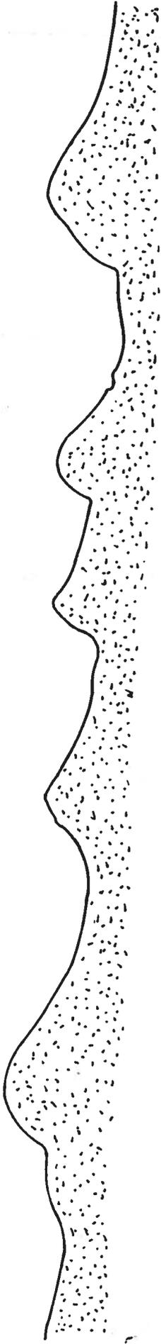
(a) PROFILE OF RIPPLED SURFACE IN BRINE MAIN<sup>(18)</sup> —MAGNIFICATION x 10
