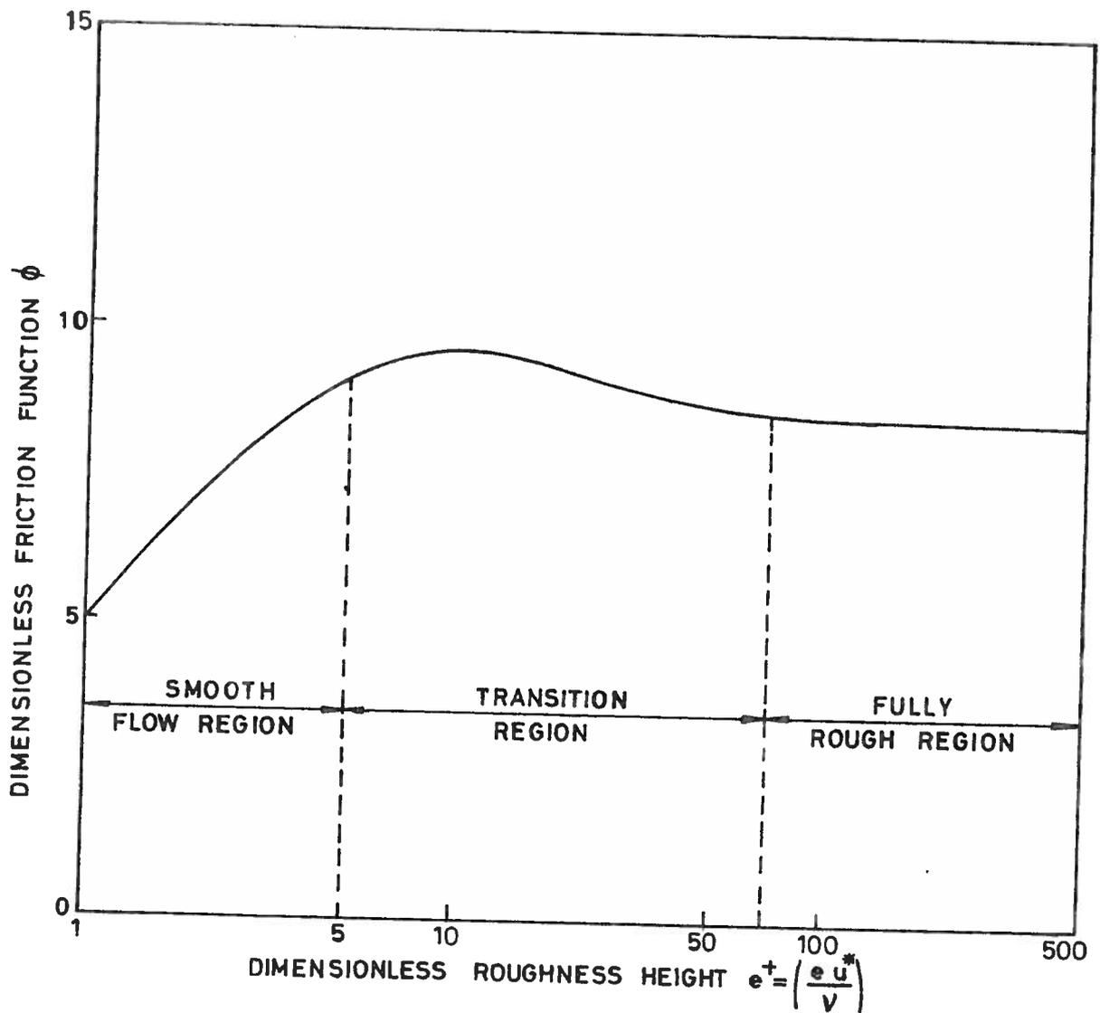
A.E.R.E.R.8703.FIG.3. CURVE RELATING FRICTION FUNCTION  $\phi$  AND ROUGHNESS HEIGHT  $e^+$  FOR ALL SAND GRAIN SURFACES—BASED ON DATA OF NIKURADSE <sup>(21, 23)</sup>
