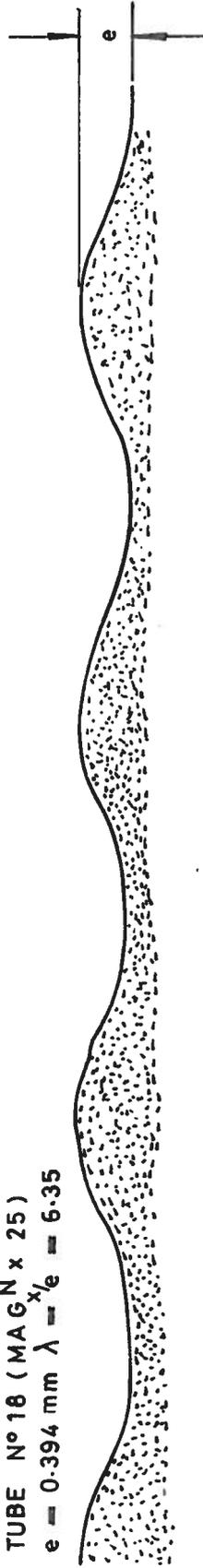
A.E.R. R.8703. FIG.10. PROFILES OF SOME SIMULATED RIPPLED TUBULAR SURFACES
