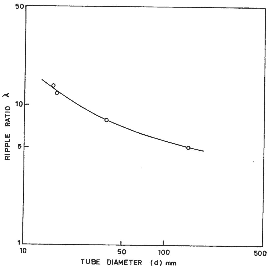
A.E.R.E. R.8703. FIG.13. ACTUAL RIPPLE RATIO VS TUBE DIAMETER FOR BOILER TUBES.
