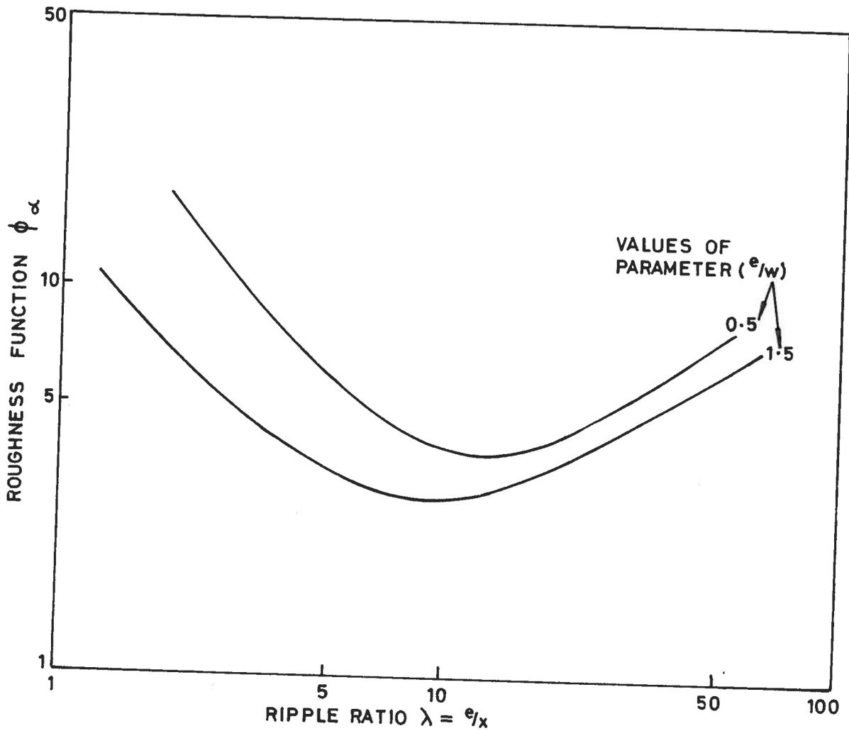
A.E.R.E. R.8703. FIG.5. ROUGHNESS FUNCTION RELATIONSHIP DERIVED BY BAUMANN AND REHME<sup>(22)</sup> FOR RECTANGULAR ROUGHNESS SHAPES— VALID FOR  $e^+ \geq 100$ .
