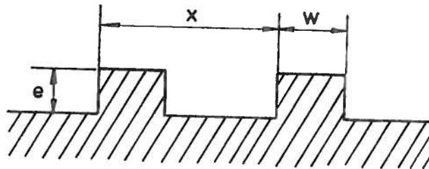
A.E.R.E. R.8703. FIG.4. GEOMETRY OF RECTANGULAR ROUGHNESSES STUDIED BY BAUMANN AND REHME <sup>(22)</sup>
