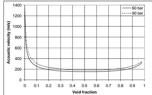
Figure 2: Speed of sound (acoustic velocity) in a gas-oil mixture at 60 bar and 90 bar.
