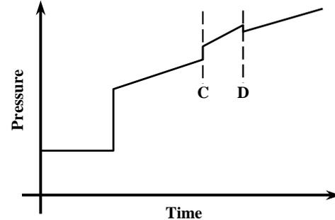
Figure 3b: Pipeline diameter reduced in interval C-D.
