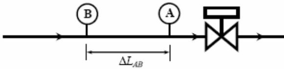
Figure 1a: Pressure pulse set-up for pipeline showing quick-acting valve and pressure transducers.
