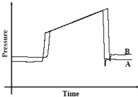
Figure 1b: Pressure pulse at locations A and B up-stream of quick-acting valve.
