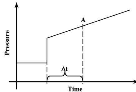
Figure 3a: Line packing increases linearly with time.
