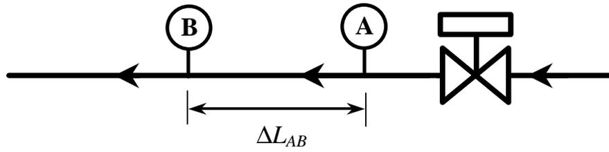
Figure 1c – Pressure pulse set-up for a gas injection line, showing quick-acting valve and pressure transducers.
