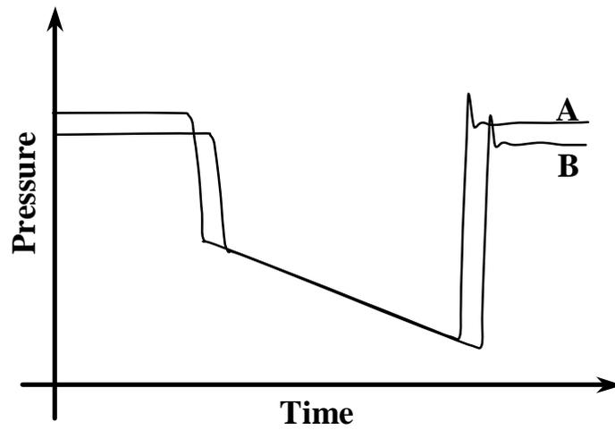
Figure 1d – Pressure pulse at locations A and B down-stream a quick-acting valve.
