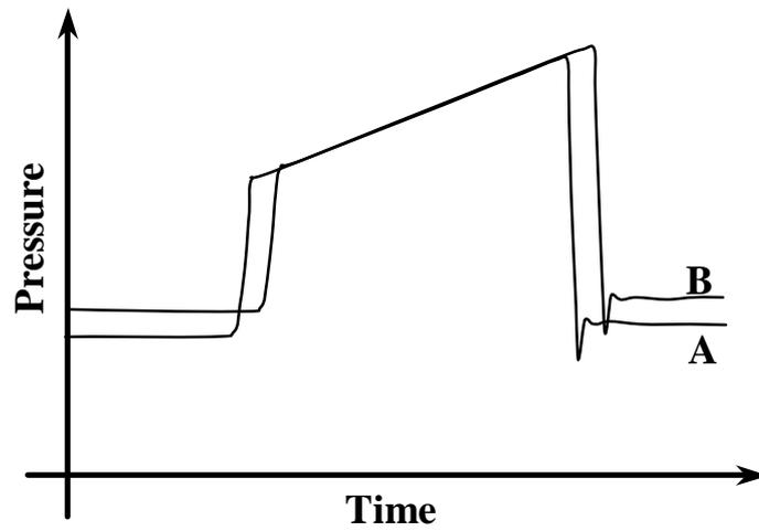
Figure 1b – Pressure pulse at locations A and B up-stream a quick-acting valve.
