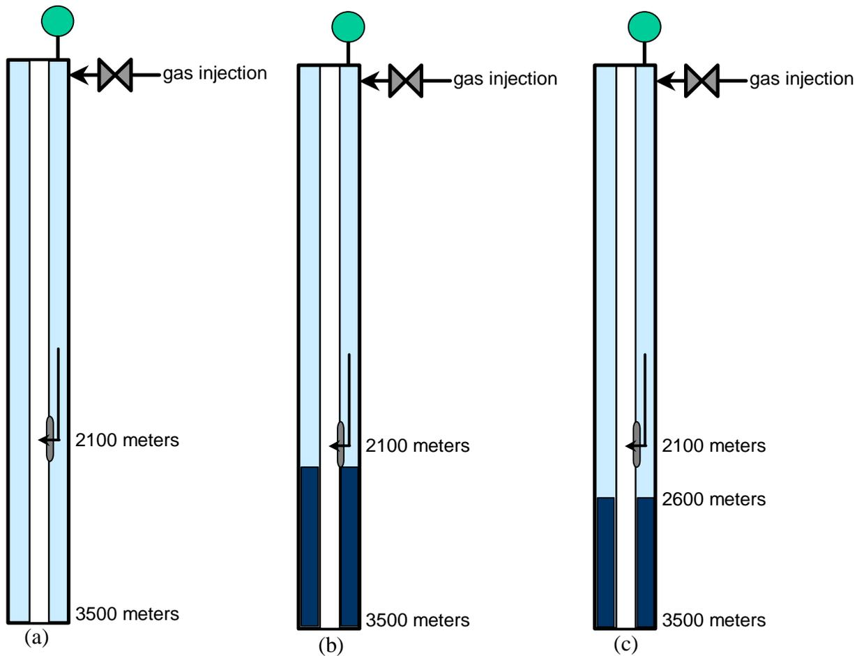
Figure 8 – Gas injection with three liquid level cases (well A)
