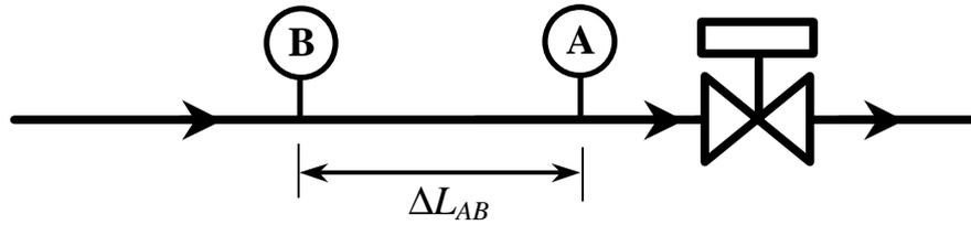
Figure 1a – Pressure pulse set-up for a pipeline, showing quick-acting valve and pressure transducers.
