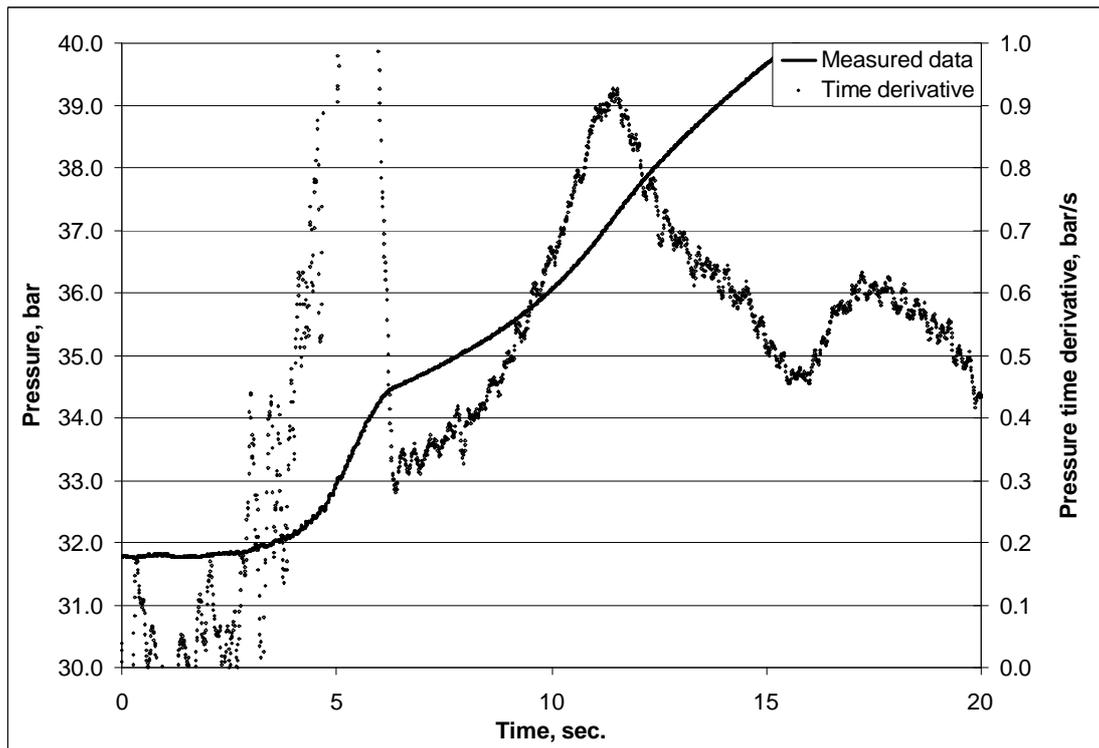
Figure 4 – Pressure pulse test on a North Sea well: The bubble point is the peak appearing at approximately 11 seconds on the pressure derivative curve.
