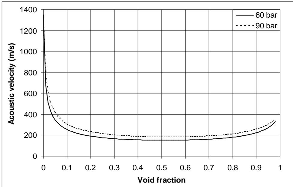
Figure 2 – Speed of sound (acoustic velocity) in North Sea production gas-oil mixture at 60 bar and 90 bar.
