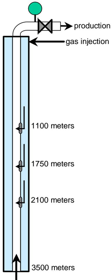
Figure 5 – Gas lift well used in pressure pulse simulations (well A)
