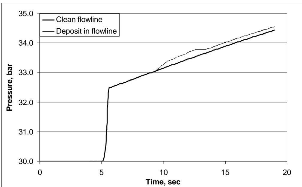
Figure 3 – Pressure pulse used to detect pipe deposits. Change in simulated response between pipe with deposits (thin-line) and clean tubing (solid-line) for the same flow rate.
